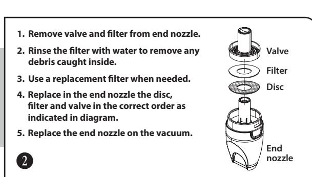
After use, always drain water from the unit by removing the nozzle and dry it before storing.
