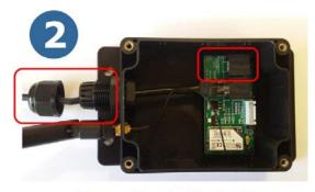
Remove lid and cable gland from SpaLINK Module
