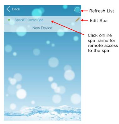
When you first complete the setup process of adding a spa it will take a few minutes for the SpaNET WiFi module to login to your wireless router, obtain an IP address and register itself on the Internet and show the spa as online. Please just wait and press the refresh button every now and then until the spa shows as online. If the spa fails to show as online after 5 minutes refer to the Troubleshooting Spa/WiFi Module Configuration on the following page.
