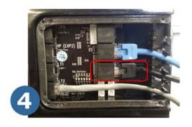
Connect black data cable from SpaLINK module into EXP1 socket
