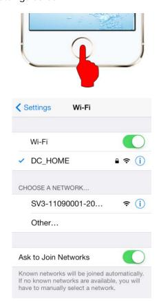
**Step 8:** Select and connect to the SV WiFi network denoted by your SV controller's serial number. No password is required to connect.
