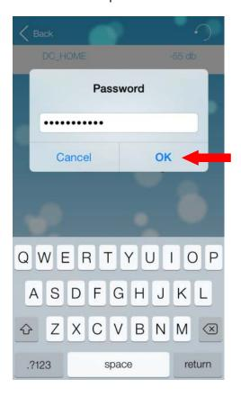
**Step 13:** Press OK to confirm the wireless network settings (SSID & Password) have been saved to the SpaNET WiFi module
