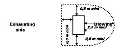
Do not to install the Heat pump in a confined place (the fan would recycle its air and the Heat pump would be down performance).
